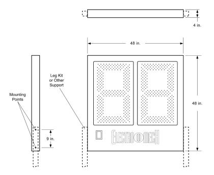
If you wish to attach your play clock displays to a different support structure, you may take advantage of the mounting plates included in the cabinets. These plates have tapped holes, spaced nine inches center-to-center, along the sides of each cabinet. The tapped holes accept 1/2-inch-13 threaded bolts. For Model LX3030, support brackets or posts would need to be positioned 48 inches apart (inside spacing) to provide room for the cabinet.
