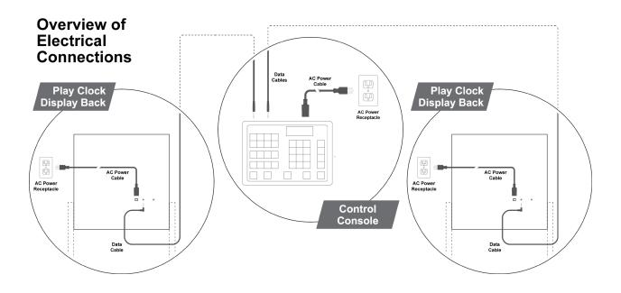
Each play clock cabinet requires a standard power receptacle. If you prefer, you may use a drop cord to bring power to the displays. Electro-Mech provides a detachable power cord with GFCI safety circuitry for each portable display. Plug these cords into the AC power sockets on the backs of the two play clock cabinets. We recommend testing (and resetting) the GFCI feature when you first plug the displays into power receptacles.
